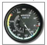
When operating on only one engine, your target airspeed should be *Vyse*, which is the speed for "best rate of climb with a single engine." Vyse is designated on the airspeed indicator with a blue radial line and often referred to as "blueline."
